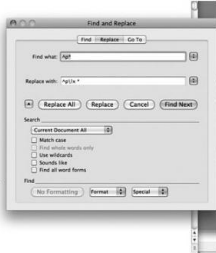
Figure 4.8. Limited regular expression search in MS Word, inserting '\lx' before each headword in a document.
